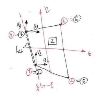
shape functions at 123:  $|V_{1}|^{2} = |V_{1}u_{2}|^{2} = 0, |V_{3}| = 0, |V_{4}| = \frac{1}{2}(1+p)$   $|U_{1}|^{2} = |V_{1}u_{2}|^{2} + |V_{2}u_{5}|^{2} + |V_{3}u_{6}|^{2} + |V_{4}u_{3}|^{2} = |V_{1}u_{2}|^{2} + |V_{4}u_{3}|^{2} = \frac{1}{2}((1-p)u_{2}+(1+p)u_{3})$ V = 2 ((1-4) V2 + (1+2) V3)
