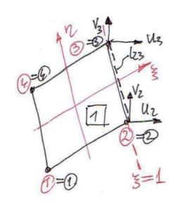
shape functions at les:  $N_1 = 0$ ,  $N_2 = \frac{1}{2}(1-2)$ ,  $N_3 = \frac{1}{2}(1+2)$ ,  $N_4 = 0$  $u = N_1 u_1 + N_2 u_2 + N_3 u_3 + N_4 u_4 =$   $= N_2 u_2 + N_3 u_3 = \frac{1}{2} ((1-\gamma)u_2 + (1+\gamma)u_3)$  $V \Big|_{23} = \frac{1}{2} ((1-12)V_2 + (1+12)V_3)$
